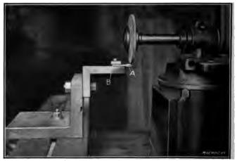
Fig. 11. Grinding Punch Sections
